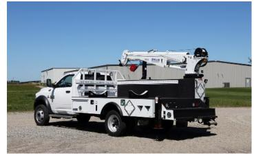
The Propane Gas Service Bodies are designed to haul a single 1000 –gallon or two 500 –gallon propane tanks, plus everything necessary to install and service the tanks. These service trucks are designed to safely carry small LP tanks with the use of E-track and fold down side rack (optional)
