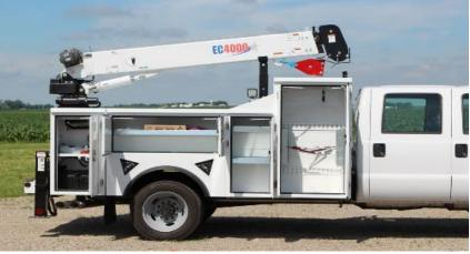
The Stellar TMAX Propane and LP Service Trucks are extremly versatile. They make transporting, loading and unloading gas cylinders a simple, single person operation without the need for a trailer or additional setting equipment. All cranes are operated with a fully radio remote control.
